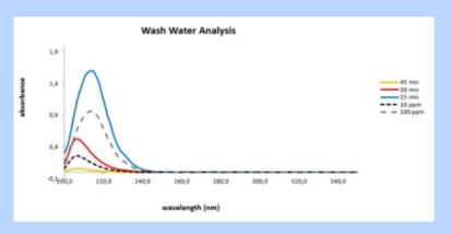
Cleaning step can be finished after 45 min. No cargo is removed anymore.
